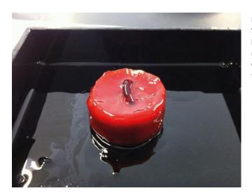
Image 2: Through liquefaction of a build volume support material drains off. © Fraunhofer ILT & Rapid Shape GmbH.
